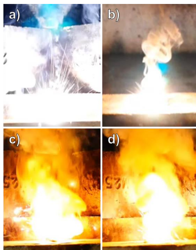
Figure 6: Still image of the flame ignition test of a) PMMA/CuO/Al (1.0 g); b) PLA/CuO/Al (0.5 g); c) PMMA/Bi 2 O 3 /Al (0.8 g) and d) PLA/Bi 2 O 3 /Al (0.8 g) thermite AM formulations
