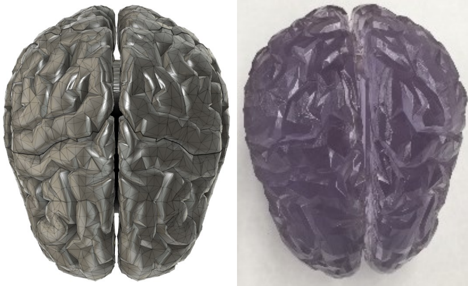
Figure 8. Numerical (left) and 3D printed (right) models of a full-size human brain
