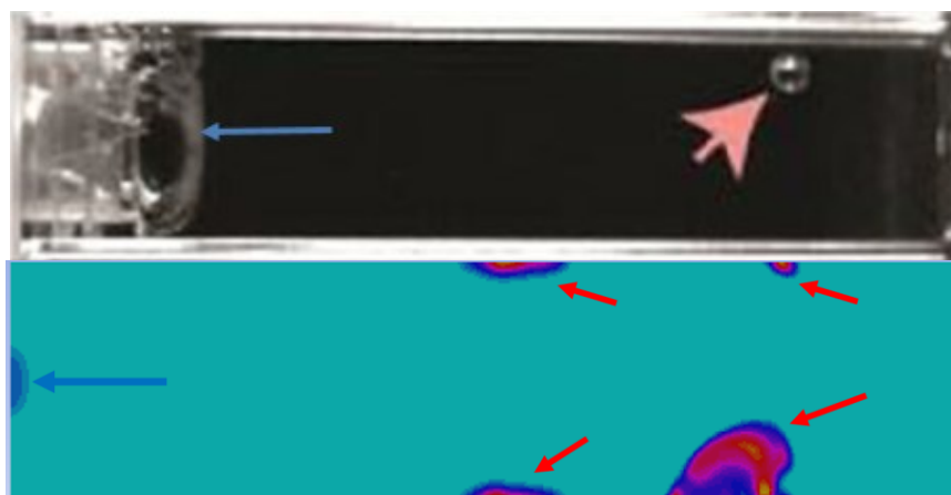
Figure 5. Cavitation (indicated by the arrows) generated in a drop test; experimental (top) and numerical (bottom).
