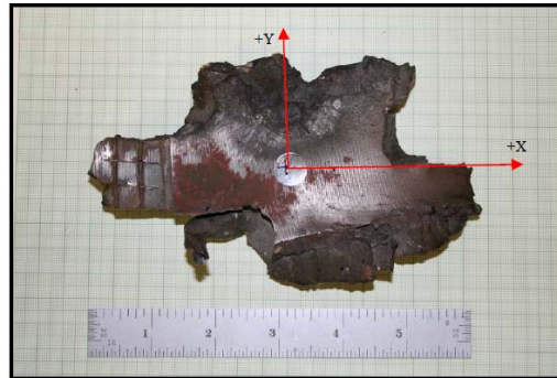
Figure 2: Fragment found at 1824 m after sub-detonative response of an artillery shell (Baker, et al. [9]).
